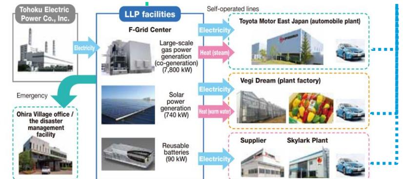
System diagram of F-grid project in Miyagi Prefecture, Japan
